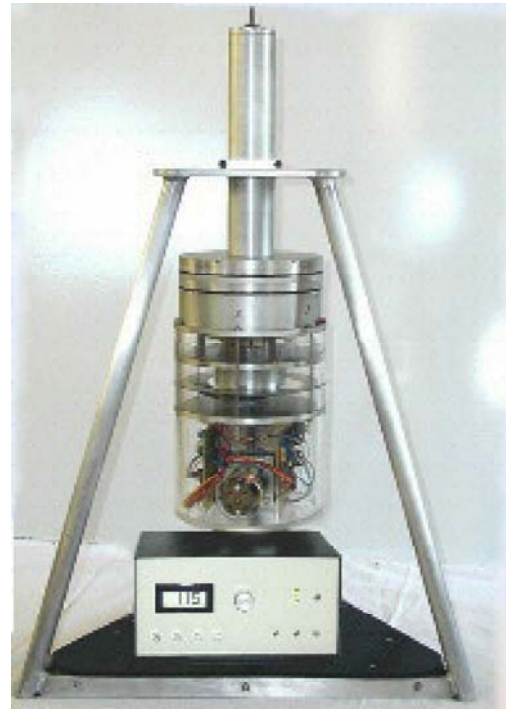
Figure 4-2 Actuator with mount and test electronics
