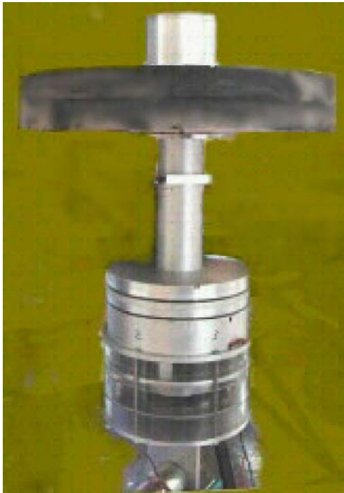
Figure 4-1 Actuator with 70 lb weight
