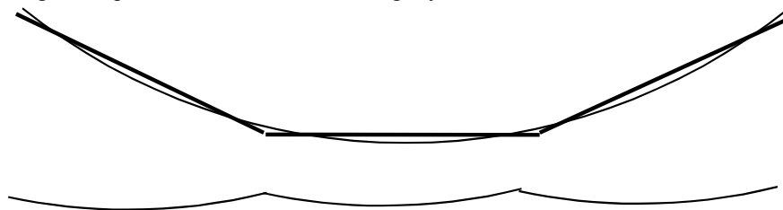
Figure 2. Illustrating the scalloped residual resulting from a faceted-approximation to a smooth aberration. The upper curve shows the uncorrected smooth aberration and the segment approximation. The lower curve shows the difference between the two.
