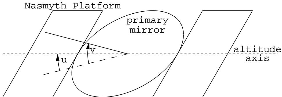
An “off-altitude-axis” position on the Nasmyth platforms brings with it three complications:
