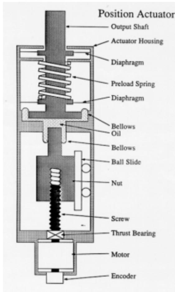
Figure 6. Schematic of the actuator design for the Keck telescopes
