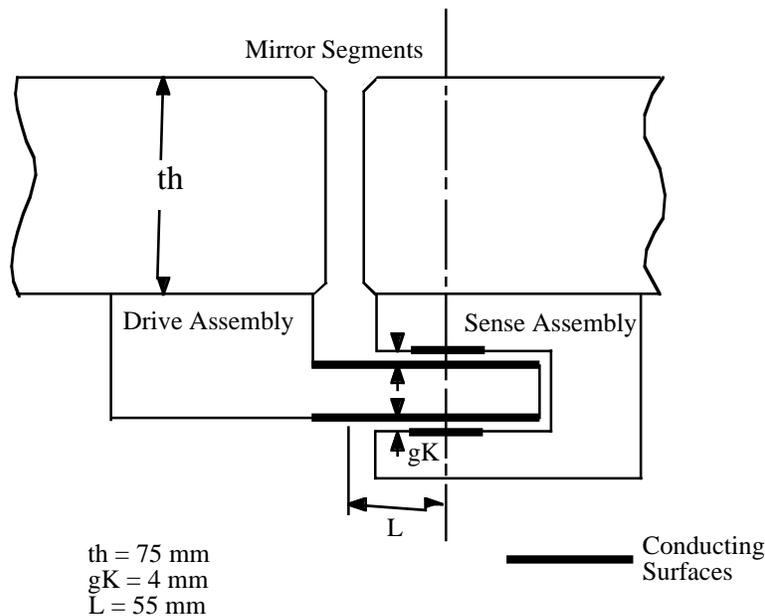
Figure 2. Schematic drawing of the Keck displacement sensor. The reflecting surfaces of the 75-mm-thick segments are at the top of the figure.
