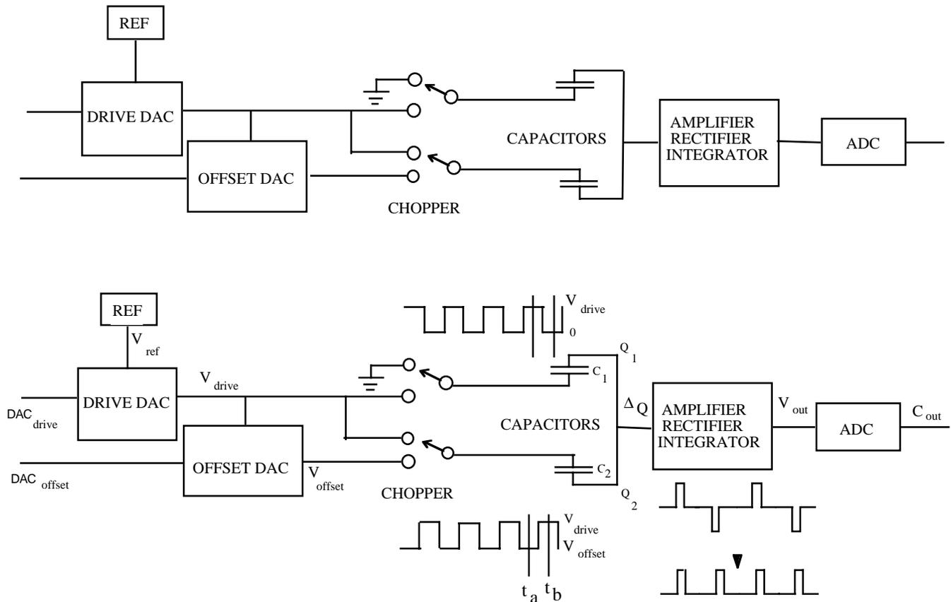
Figure 3. Schematic of the Keck sensor electronics functions.
