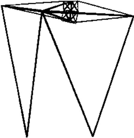
Fig. 2(b) - Model S.2 - Mode shape for  $f_n = 2.74$  Hz
