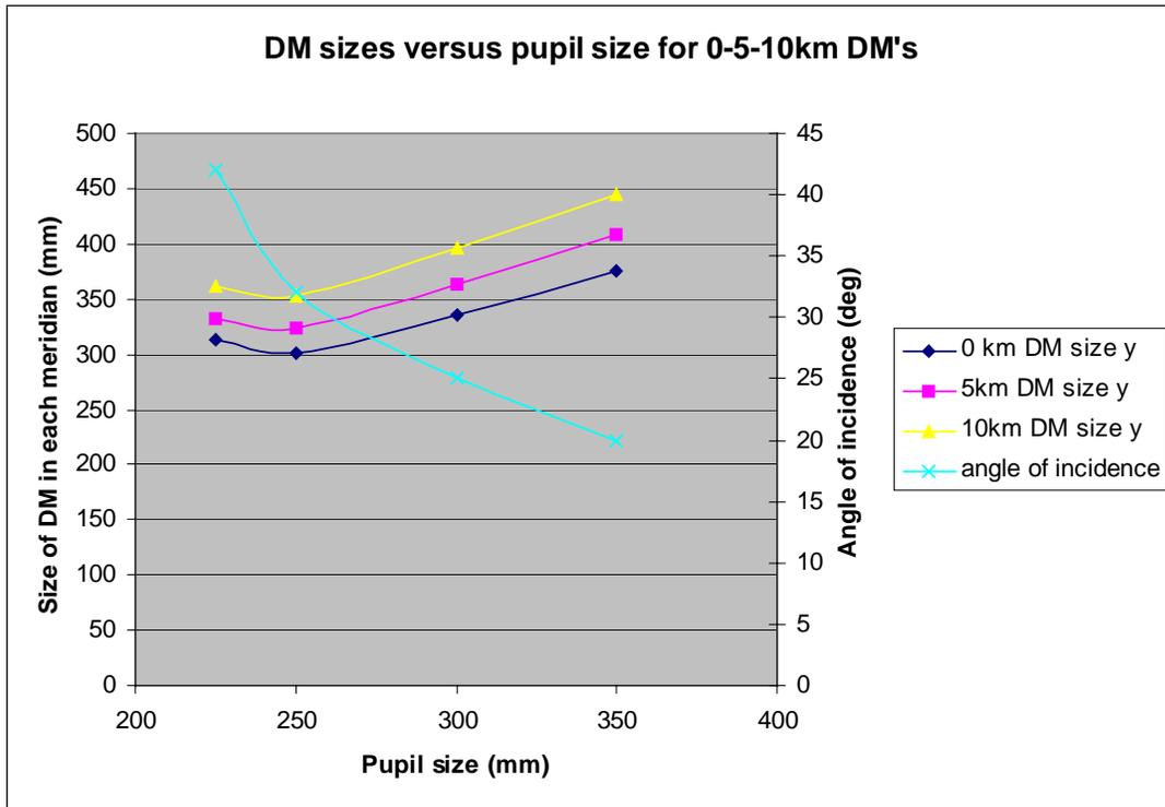
**Figure 1.** Deformable mirror diameter for three conjugate locations in a collimated space. The 0 km conjugated mirror is the smallest diameter while the 10 km conjugated mirror must increase in diameter to accept a field angle (in this case) of 2 arcmin diameter. For small pupil sizes, the packaging of three mirrors in a small space leads to the increasing mirror diameter. (The placement of three DMs in a diverging beam leads to a similar curve, but all mirror diameters can be made equal.)
