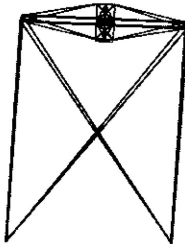
Fig 1(b) Model S.1 - Mode shape for  $f_{min} = 4.05 \text{ Hz}$
