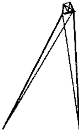
Fig. 7(b) - Model T2 Mode shape for  $f_{n=1} = 4.12 \text{ Hz}$
