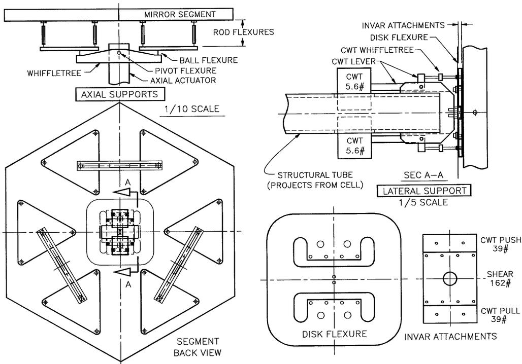
The distortion of the segment due to this support was calculated to be 10.5 nm p/v, with an rms of 1.8 nm.
